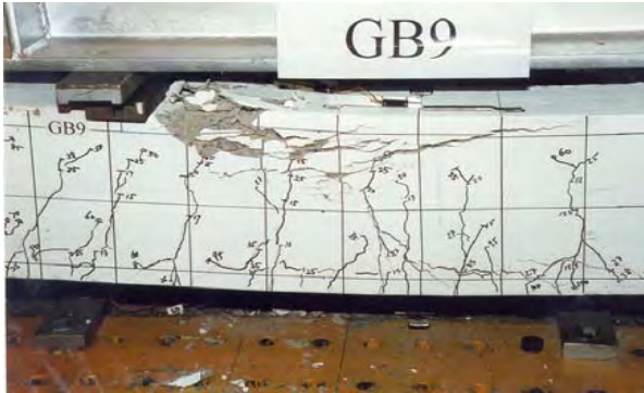
Flexure and Cracking
