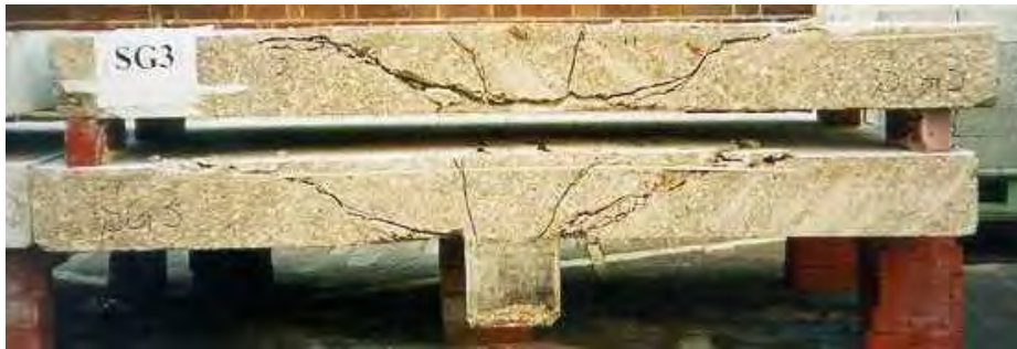
Section through Slab SG3 at Failure
